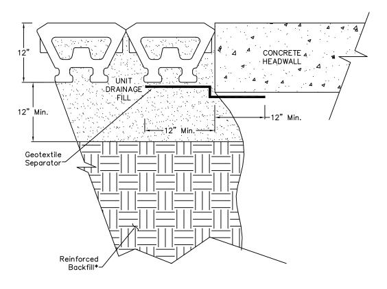
\*Reinforced backfill shall be drainage stone to an elevation which is equal to or above the expected high water elevation unless otherwise specified in the final design drawings.
